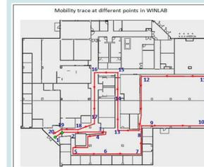
➤ Measured signal strength of different APs by moving inside different locations of WINLAB (left).
